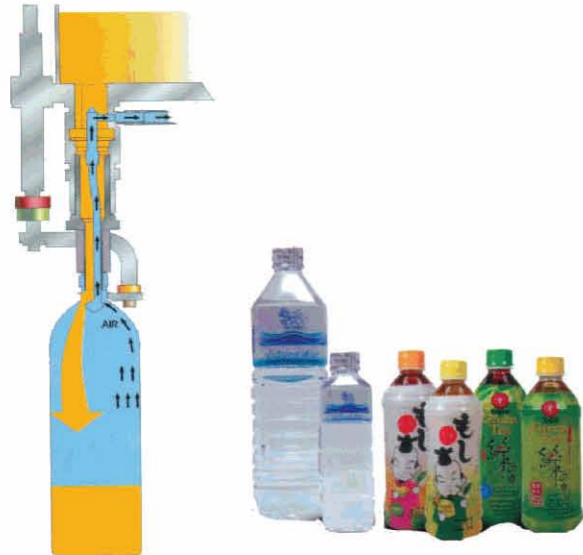
MONOBLOCK TYPE RINSER / FILLER / CAPPER CAPACITY - 38000 BPH (For 600 ML MINERAL WATER)
